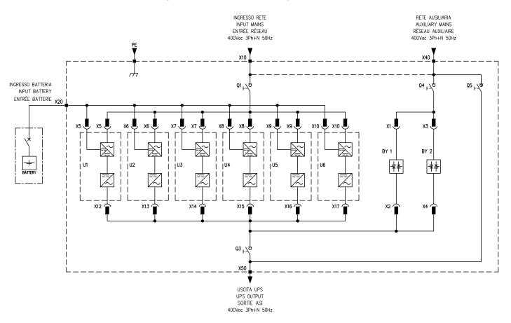
System with manual bypass, input, aux. mains and output switches and internal backfeed (with or without redundant bypass module).
