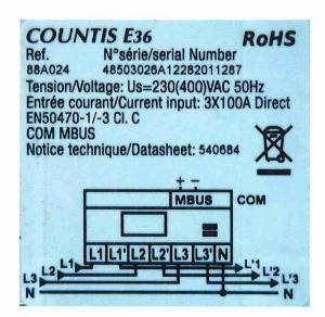
Figure 2 – Examples of type plates
