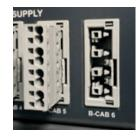
Figure 14. B-Cab aux supply connectors
