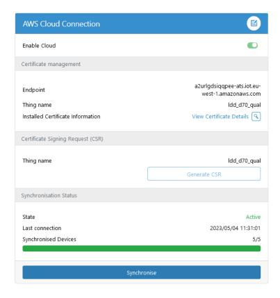
After few seconds, the gateway should connects to AWS and synchronize devices. You should be able to see uplinked MQTT messages in the AWS MQTT Test Client.
