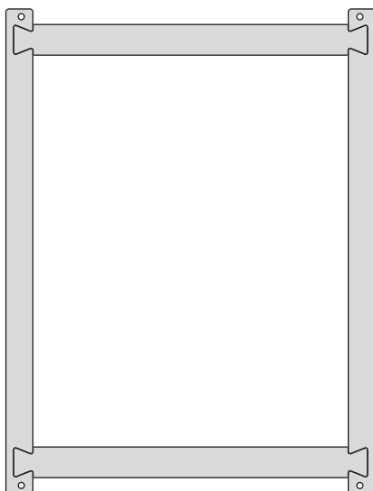
Figure 28. Holes to drill for 1 C-Cab installation
