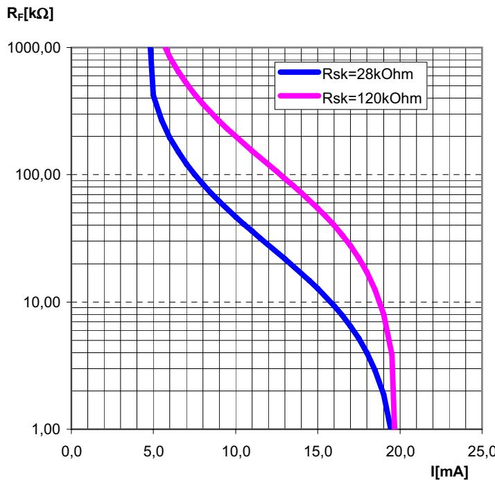
$$R_F = \frac{16 \text{ mA} \times R_{Sk}}{I - 4 \text{ mA}} - R_{Sk}$$
