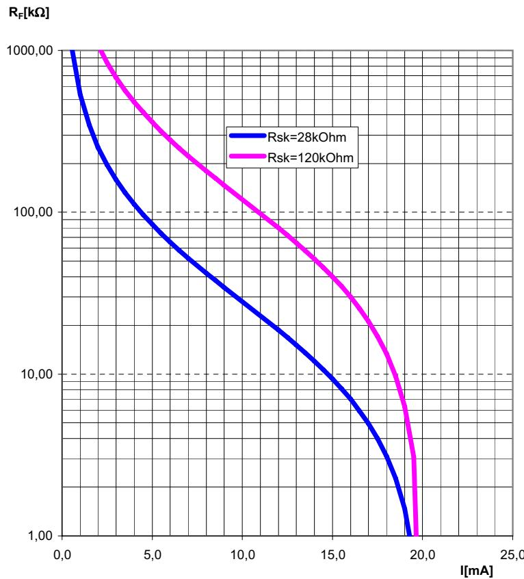
$$R_F = \frac{20 \text{ mA} \times R_{Sk}}{I} - R_{Sk}$$
